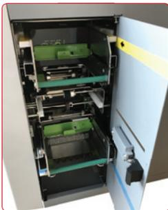
The metal cover on the side of the dual feeder allow easy access to the removable cartridges.
